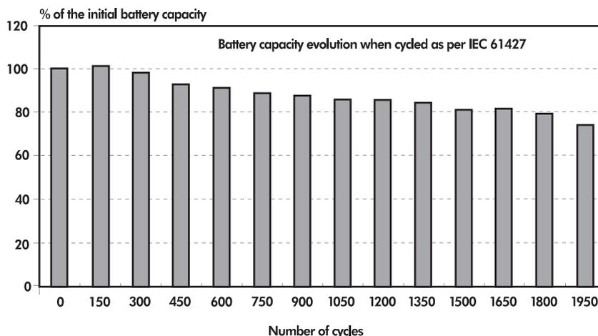
Figure 5 – Alcad Solar cycling to IEC Standard 61427
