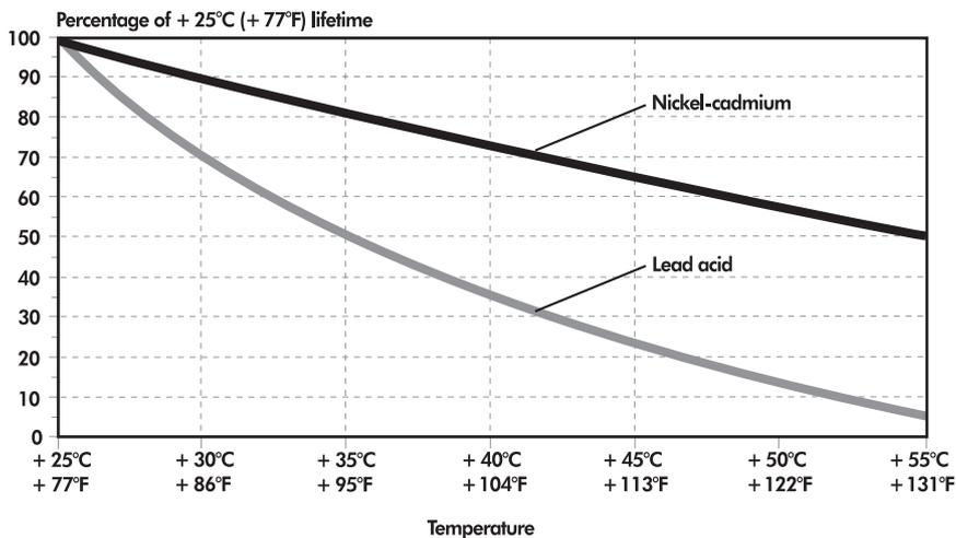
Figure 6 – Lifetime reduction with temperature
