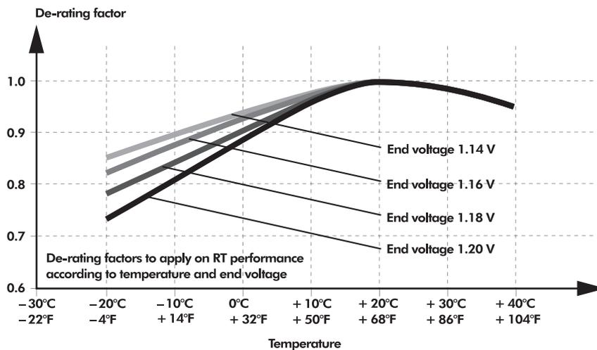
**Figure 1 – Temperature de-rating: standard electrolyte for operating temperatures from  $-20^{\circ}\text{C}$  to  $+40^{\circ}\text{C}$  ( $-4^{\circ}\text{F}$  to  $+104^{\circ}\text{F}$ )**
