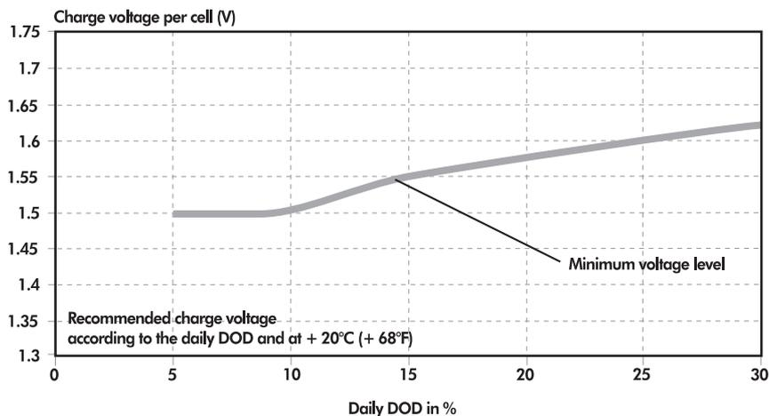
Figure 7 – Charge voltage required for high state of charge
