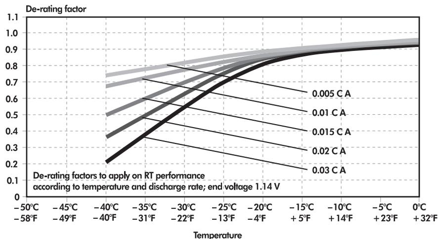
**Figure 2 – Temperature de-rating: special electrolyte for operating temperatures down to  $-40^{\circ}\text{C}$  ( $-40^{\circ}\text{F}$ )**
