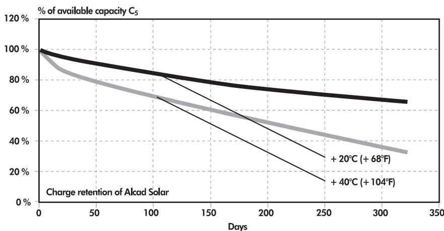
Figure 3 – Open circuit loss at +20°C and +40°C (+68°F and +104°F)
