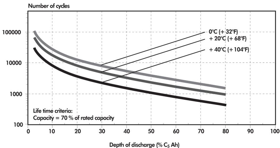
Figure 4 – Typical cycle life values at different temperatures
